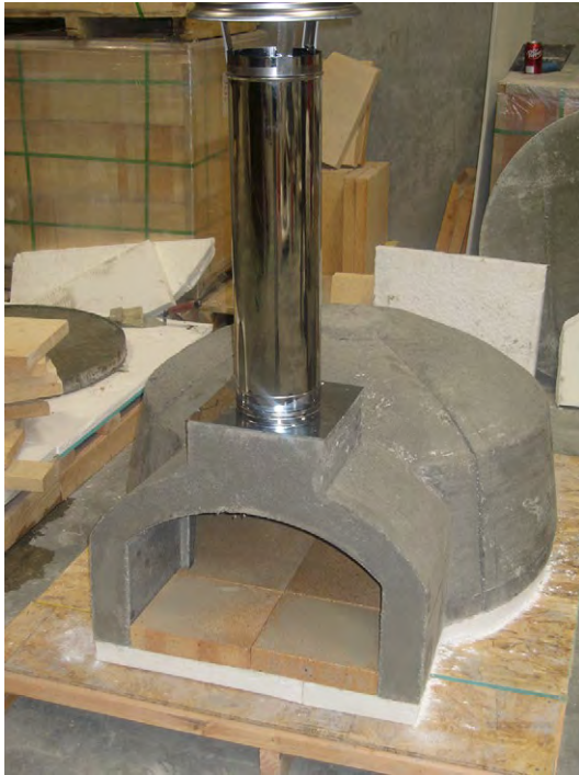
6.1 Casa2G with single wall stainless steel chimney.
